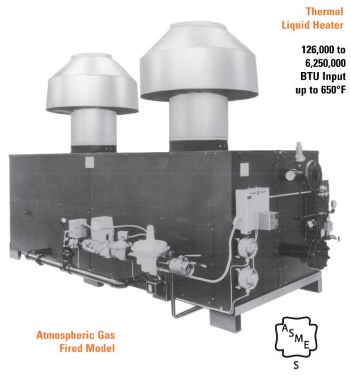
Correctly engineered, a Thermal Liquid System is extremely trouble free. Operating pressures are very low permitting the use of standard pipe and fittings. The entire system can be open to atmosphere through the expansion tank. Thermal liquids specifically compounded for high temperature service are readily available.
