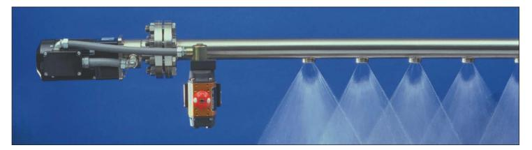
With any piping network, debris travels through supply lines, causing shower nozzles to plug. **HelioJET Fast Clean Showers**<sup>™</sup> are designed with internal rotating brushes that unplug every nozzle in a matter of seconds. This technology eliminates felt streaks and improves moisture profiles by delivering consistent pressurized hot water and He-Chem<sup>™</sup> cleaning agents evenly across the felt. Fast Clean Showers are available in manually operated, or motorized versions.
