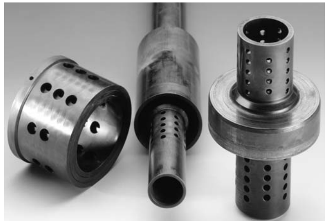
Internals of a leak-off valve ZK 213, DN 100, after 13 years of operation with p_1 = 374 bar (5420 psi), p_2 = 11 bar (159.5 psi), t = 172 °C, \dot{m} = 35 kg/s
