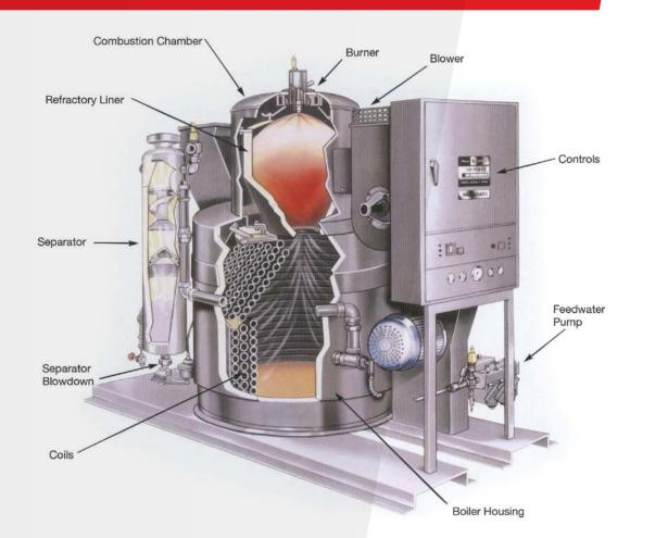
**BOILER TYPE:** Sectionalized coil tube type, forced circulation, forced draft fired.
