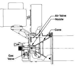
Cross sectional view of a Model "400" OVENPAK® Gas Burner
