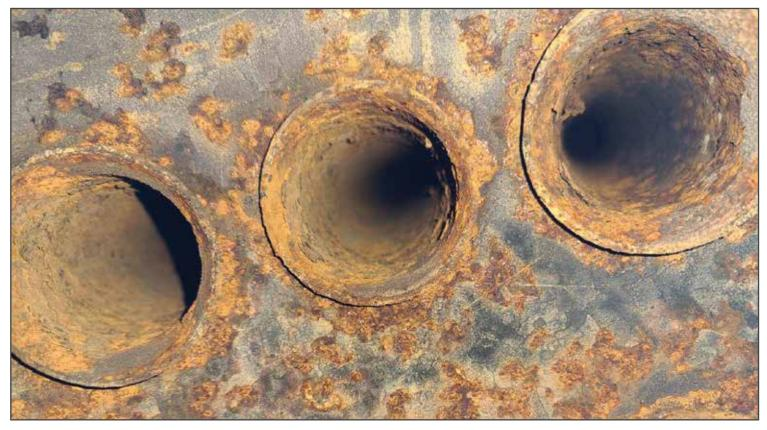
Look at an old piece of iron or steel that's been laying around a while, especially one that's been exposed to the elements. Not exactly smooth, is it? Kinda rough and pitted. As we all know, boilers are made from the same stuff. Which means they have to play by the same rules of chemistry and physics. In other words, when the metal in a boiler comes in contact with oxygen, it starts to break down and form metal oxides – also known as rust.
