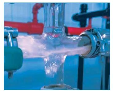
hammer effect. But water hammer can also occur if a steam pipe experiences a sudden increase in pressure. That sudden pressure increase can cause a pressure wave to travel through the pipes, which will pick up any condensate with it and smack it into the next solid surface it hits. That can sound like anything from a small rattle to a loud bang.
