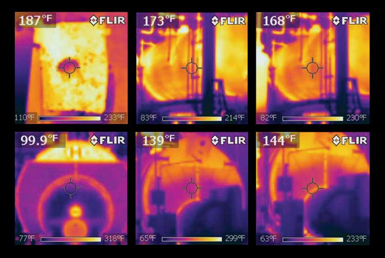
The Valve Shop uniquely incorporates utilization of infrared thermography in Steam System repair and maintenance. Using a thermal imaging camera, technicians can see variations in temperature enabling them to pinpoint hot spots and steam leaks quickly and easily. This technique can enable the technician to find problem areas in your system that can't be seen by the human eye and fix them before they become a major issue.
