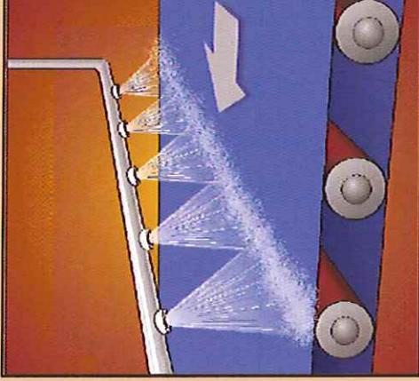
clean the machinery without negatively impacting the consistency of the paper with excess water. The results are less wasted product and decreased down-time from having to stop the production process and clean the equipment when quality problems arise.
