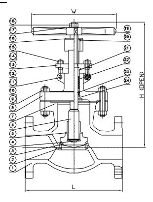
Davis cast steel valves comply with the following applicable specifications: ANSI B16.10, ANSI B16.5, API 6D: Tested to API 598
