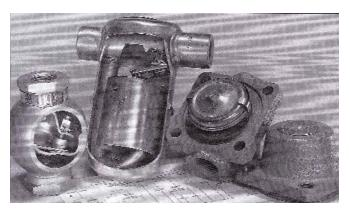
L to R - Adjustable Bimetallic trap, Inverted Bucket trap, Balanced Pressure Thermostatic trap
